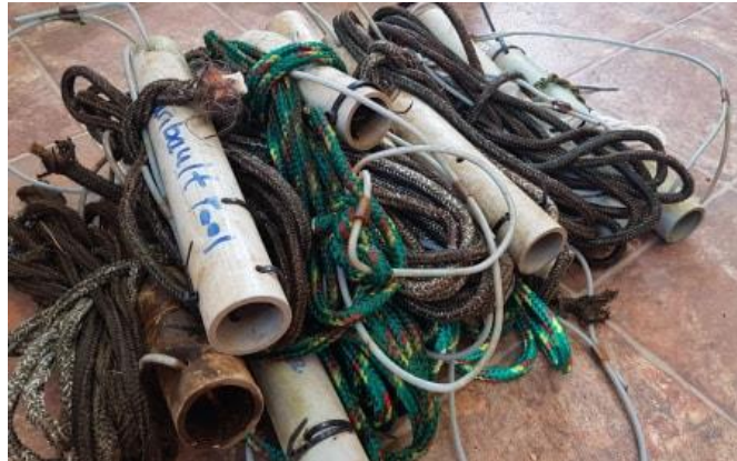
Figure 1: The housing for CRSA’s water temperature loggers used in the 2019 study period.
