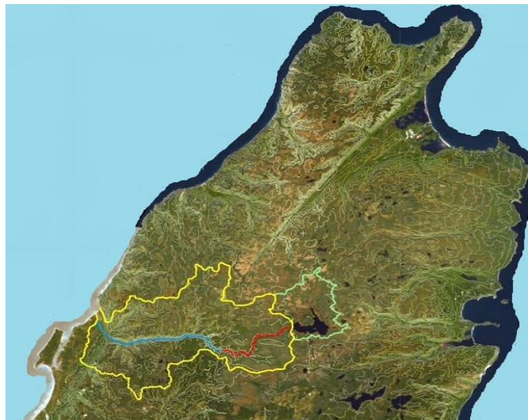
Map showing watershed boundaries for the Cheticamp River (secondary watershed). The green boundary shows the watershed area diverted for the Wreck Cove hydroelectric project. The portion of the river coloured in red indicates where there is no fish passage above the barrier falls. Image credit: James Bridgland, CBHNP.
