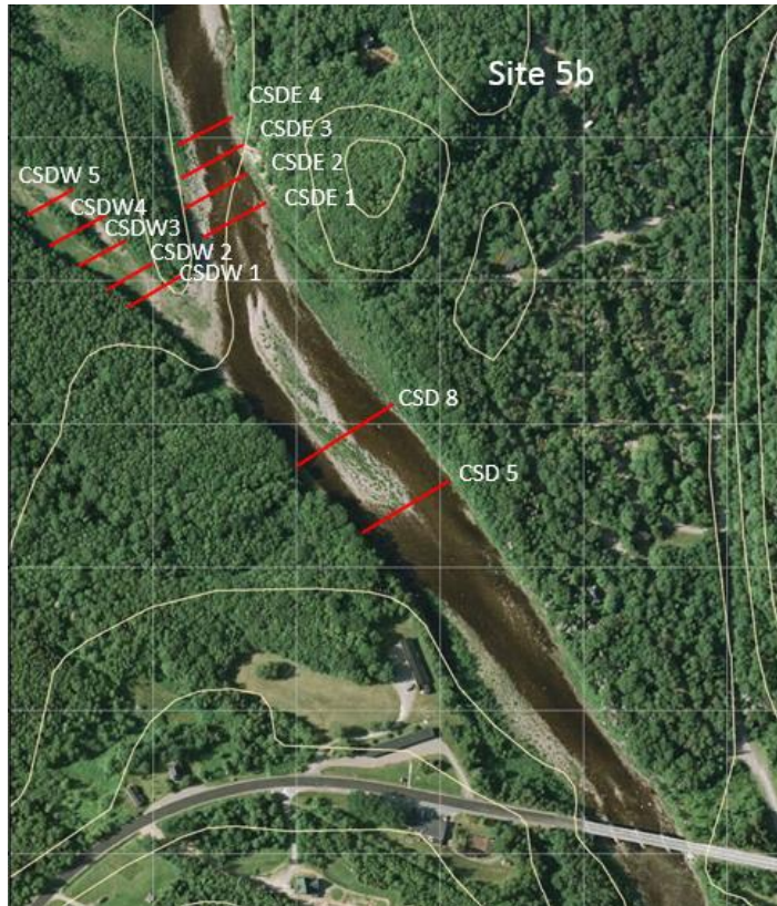
Figure 3a. Overview of cross section locations in Site 5b 2015. Note the mid-channel bar at CSD8 location is no longer present at that location but has moved downstream to plug the eastern channel
